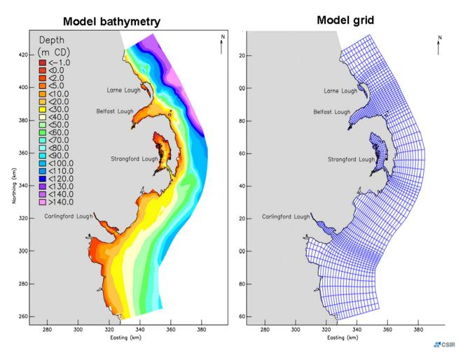
Fig. 3. Delft3D model bathymetry and grid. Note the very dense grid inside the loughs, comprising hundreds of cells and 8 sigma layers.
