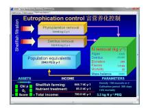
Mass balance for nutrient removal and overall water quality effects.
